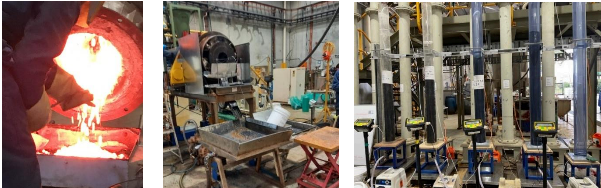
Figure 10 - Pellets being unloaded from the pot grate, pilot testwork set-up showing rotating drum and filtering operations and counter-current 1m leach column arrangement
