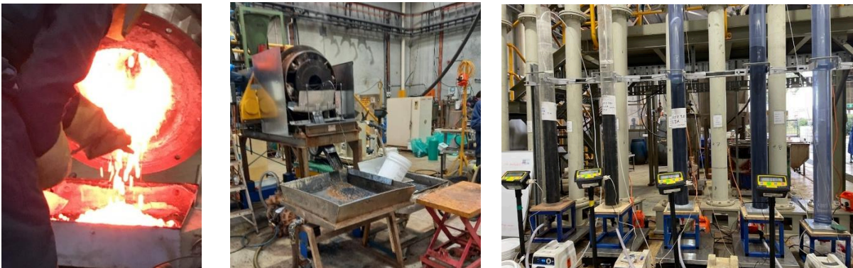
Figure 1 - Pellets being unloaded from the pot grate, pilot testwork set-up showing rotating drum and filtering operations and counter-current 1m leach column arrangement
