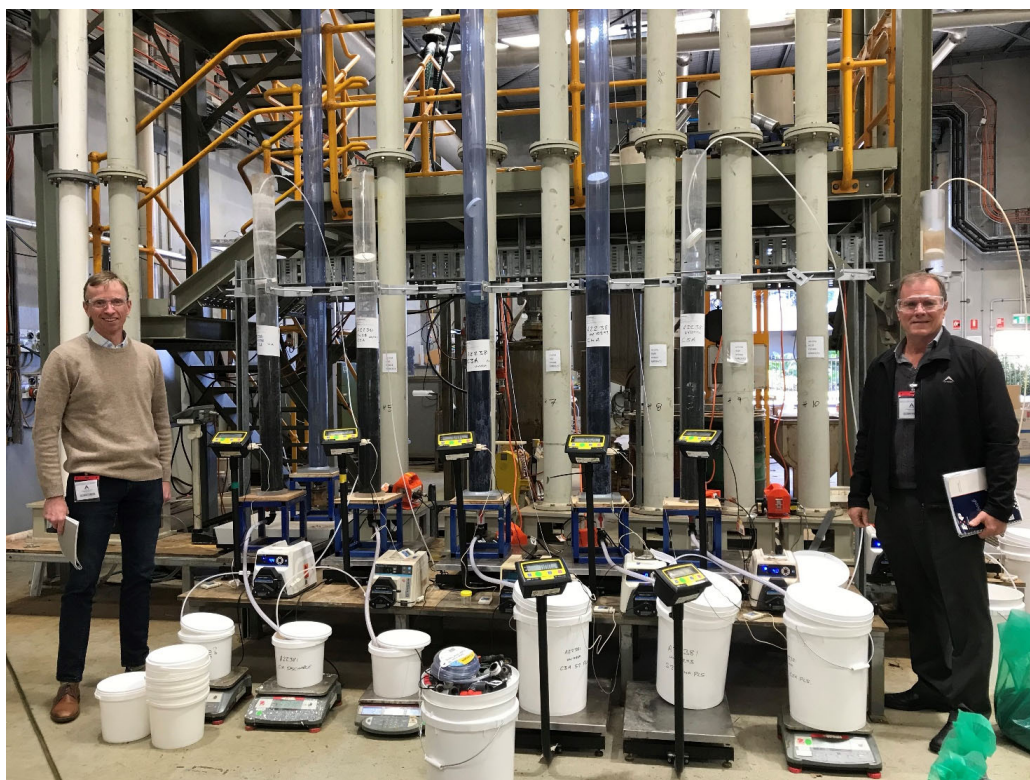
Figure 5: Process Engineer Greg O'Connor and Project Manager Trevor Smith inspecting the final stage of the heap leach test
