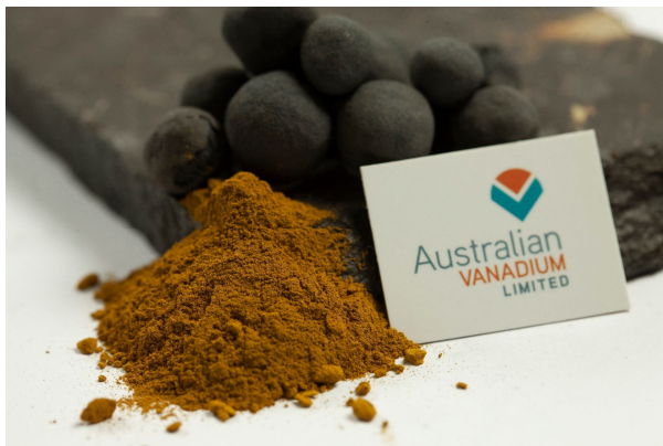
Figure 4: Sample of V_2O_5 precipitate generated from pilot program alongside roasted pellets and a vanadium ore sample.
