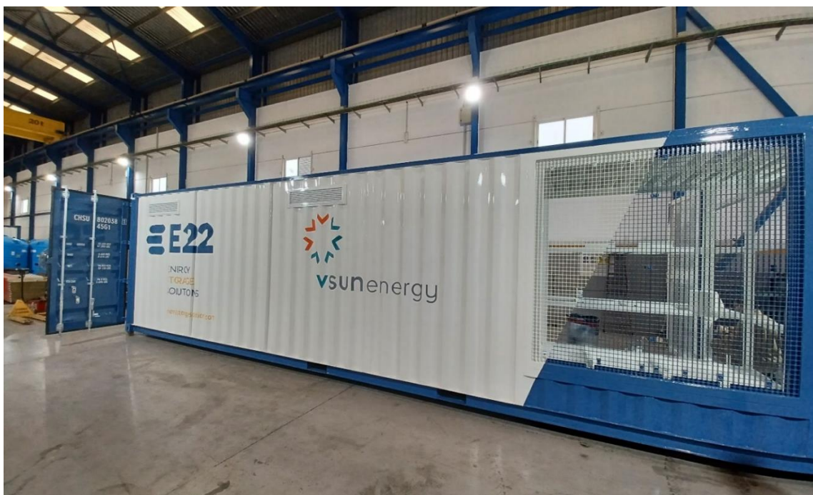
Figure 5 VRFB for standalone power system at IGO's Nova Nickel Operation under construction
