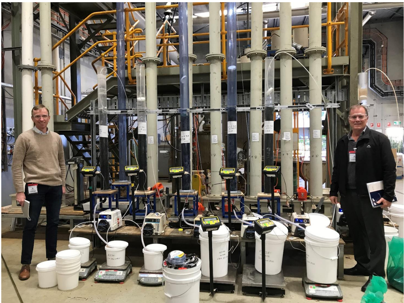
Figure 4 Process Engineer Greg O'Connor and Study Manager Trevor Smith inspecting the final stage of the heap leach test
