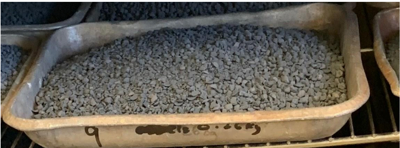
Figure 2 Pilot feed - roasted pellets crushed to <6.3mm
