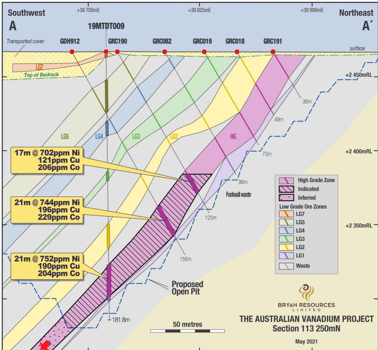
Figure 3: Cross section at 113 250 mN showing geology model and the location of the base metals Mineral Resource categories.
