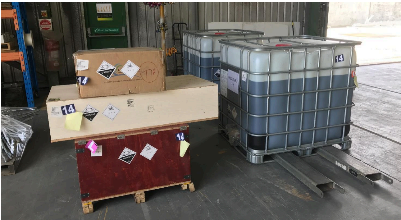
Figure 1 CEC 5kW/30kWh VRFB package with vanadium electrolyte ready for assembly and testing at CADDs Group
