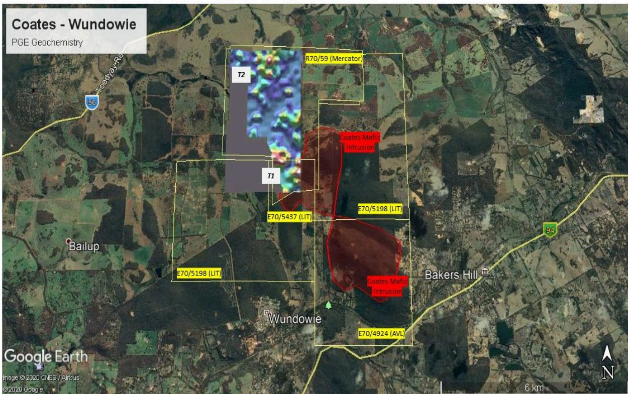
Figure 2 Pt + Pd contoured grid in NW corner of tenements from bottom of hole analysis of Bauxite Resources Limited’s vacuum drilling, showing anomalous PGEs at edge of Coates Mafic Intrusion
