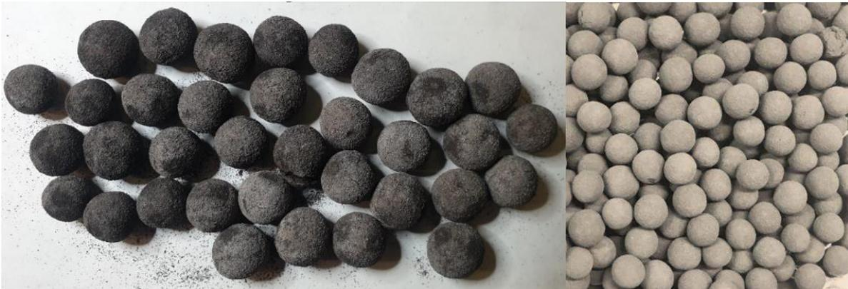
**Figure 1: Vanadium rich iron concentrate pellets produced during bench-scale roast testing**
