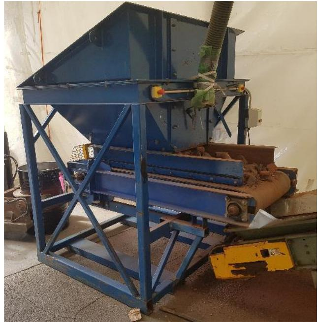
*Plate 5 Trans hopper feed to prime crusher*
