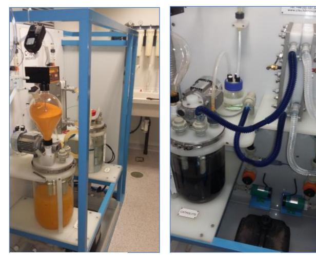
Figure 4 - Initial Vanadium dosing of Acid
