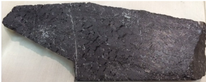
* High-grade massive V-Ti-Fe mineralisation from diamond drill hole GDH 903. Refer to full JORC Resource Table on Slide 14.
