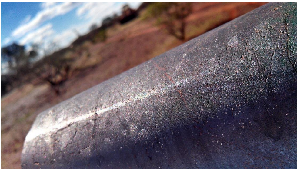
Figure 1. An image of high grade massive magnetite PQ (83mm diameter) core from Gabanintha
