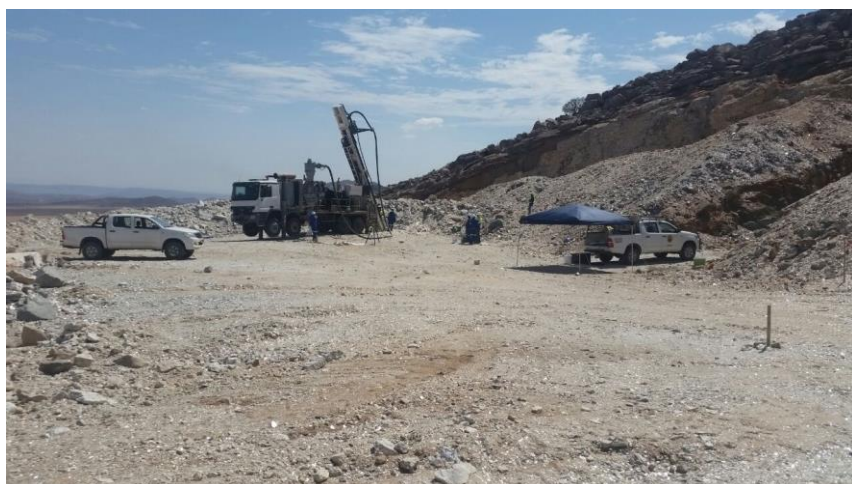
Figure 1. RC drill rig set up at BBRC001 location, Pegmatite excavation visible in background
