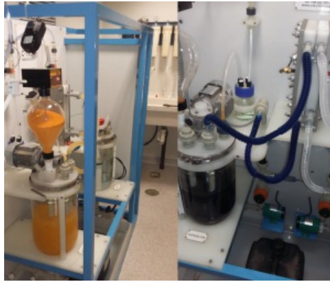
Initial Vanadium dosing of Acid; and Balanced Vanadium electrolyte
