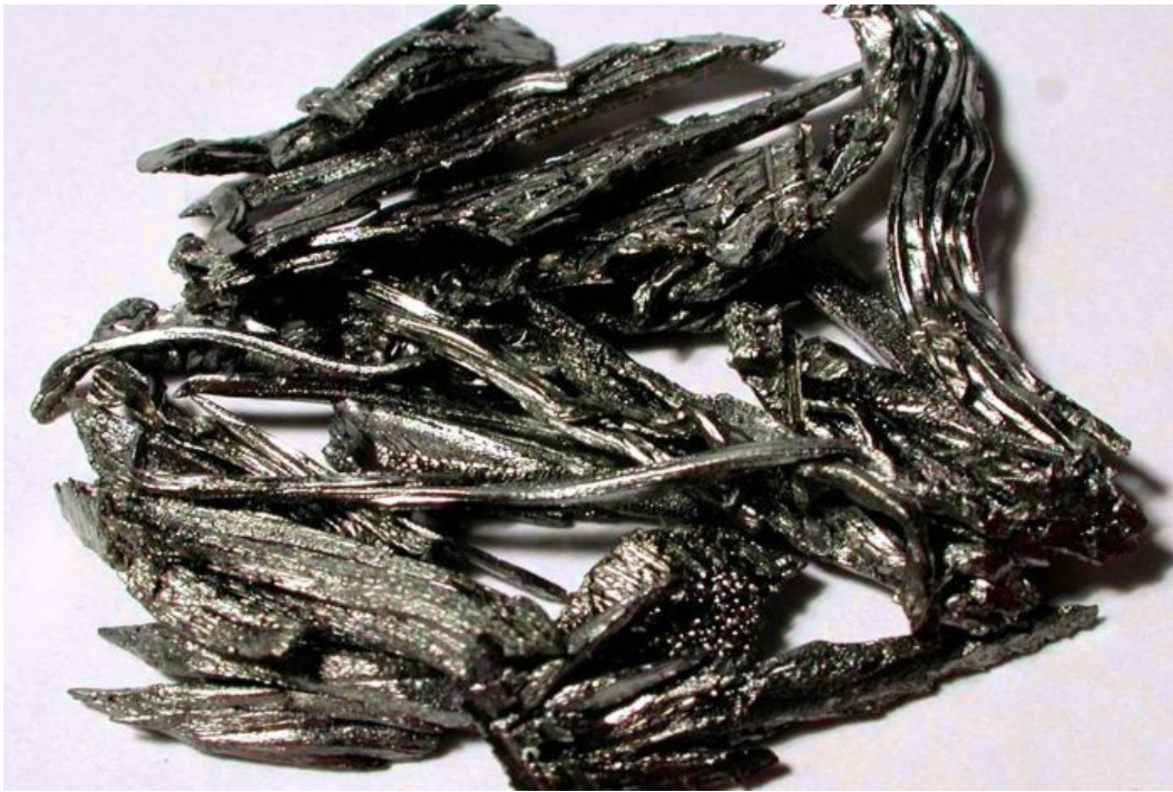
PHOTO: Dysprosium, a rare earth element used in magnets for electric vehicle motors, is resistant to demagnetisation at high temperatures. (Supplied: Northern Minerals)
